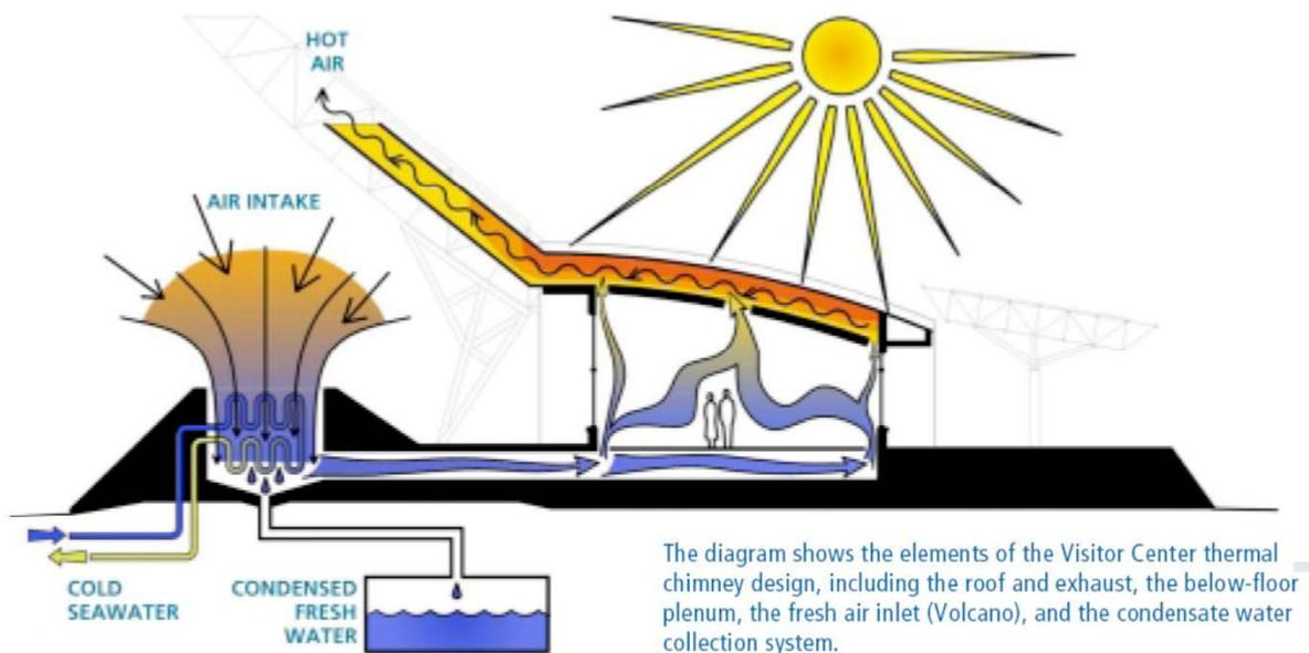
Figure 6. The Deep Seawater cooling system at the Hawai'i Gateway Energy Center. Figure by Ferraro Choi Architects.
