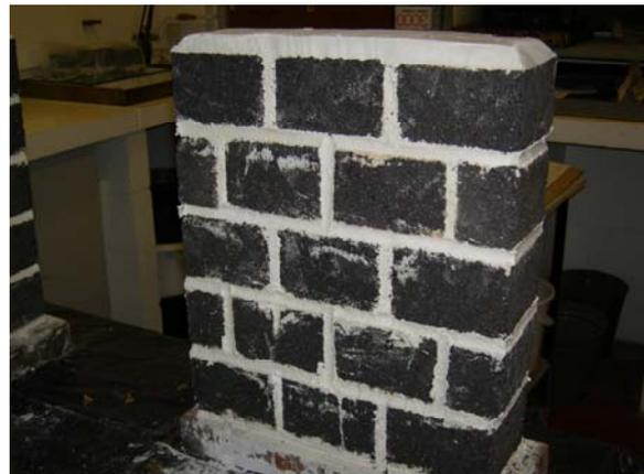
**Figure 5.** Bitublock Wall (un-cleaned)
