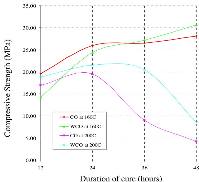
**Figure 2.** Effect of cure duration and temperature on compressive strength
