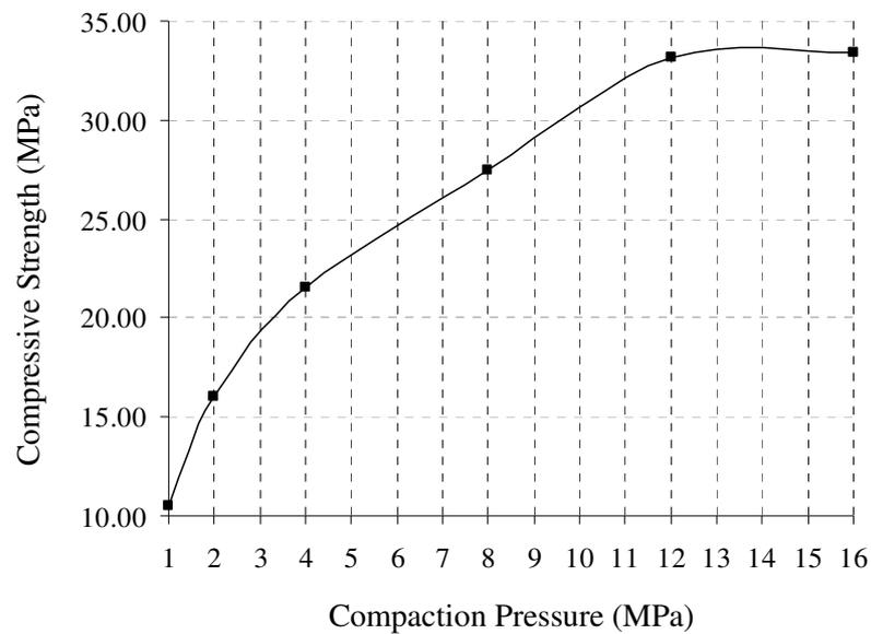
**Figure 3.** Effect of compaction level on compressive strength
