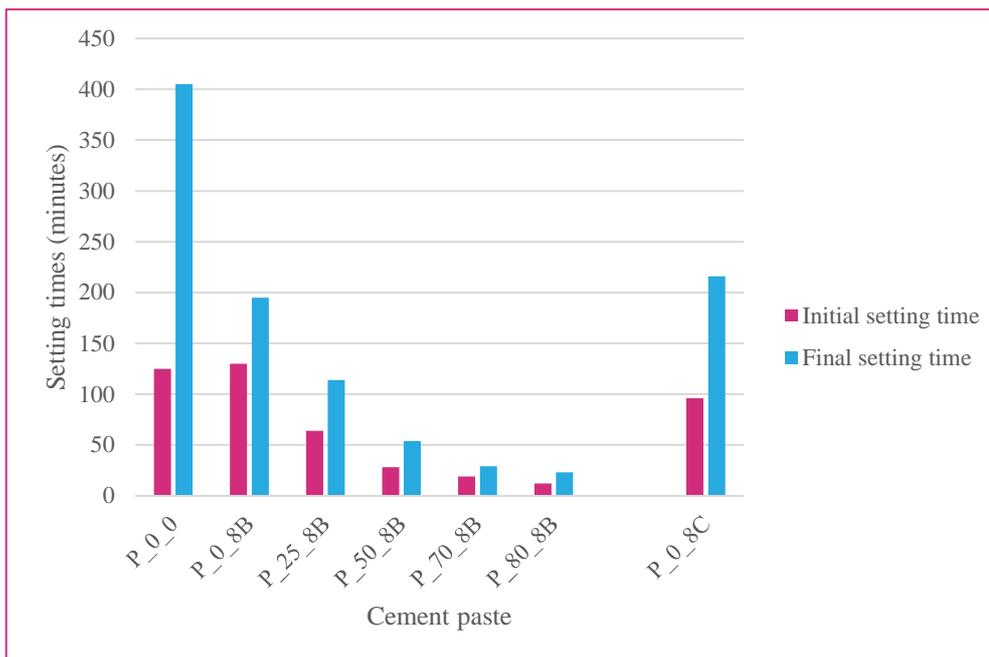
**Figure 4: Setting times for pastes accelerated with CSA powdered accelerators**
