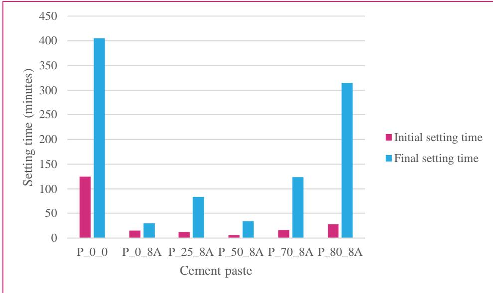
**Figure 3: Setting times for pastes accelerated with liquid alkali free accelerator**
