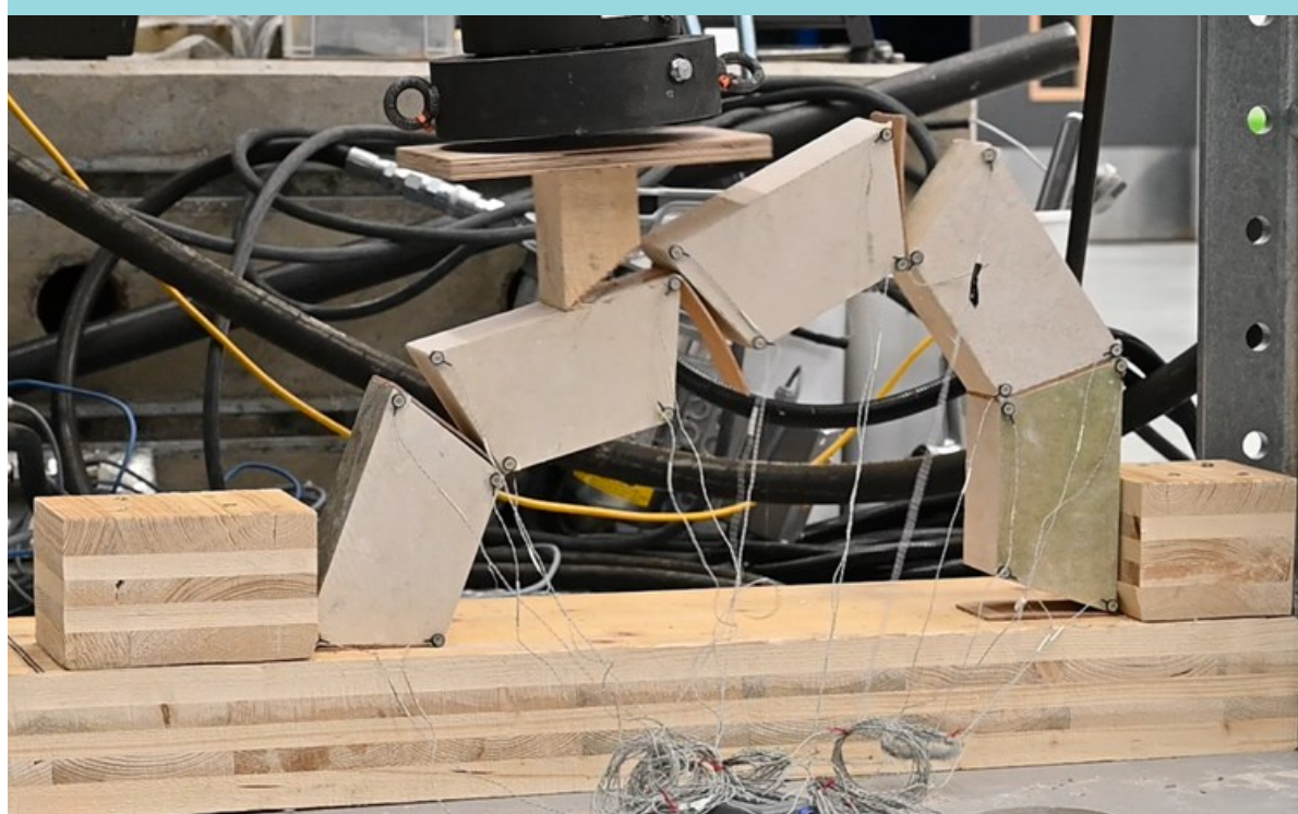
Cork arch on the point of collapse
