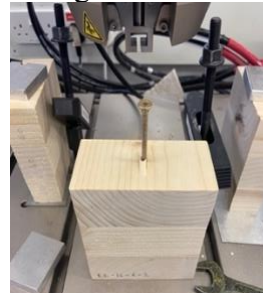
Withdrawal Failure 6mm/min
