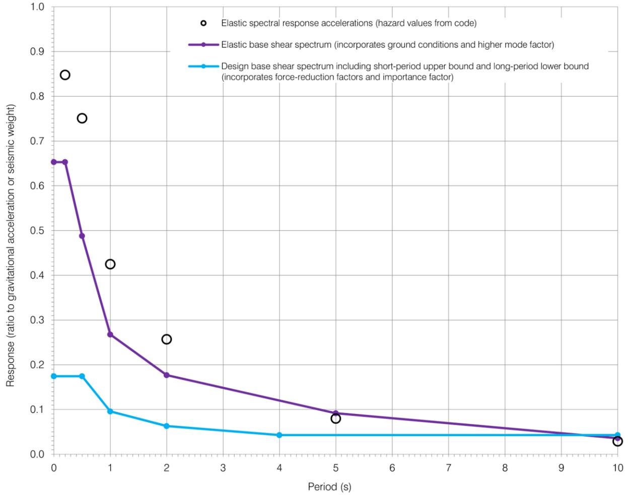
Example spectrum for Vancouver and site class B, for a normal importance concrete shear wall building with  $R_d = 2.0$  and  $R_o = 1.4$
