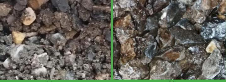
Figure 3. Uncoated and coated aggregate after sulfate soundness test
