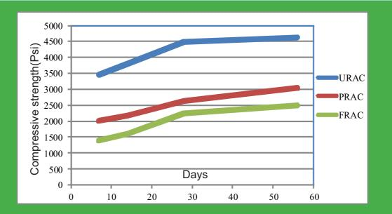
There is week bond between PCRCA and cement paste in concrete leading to a low strength of concrete than uncoated RCA concrete.
