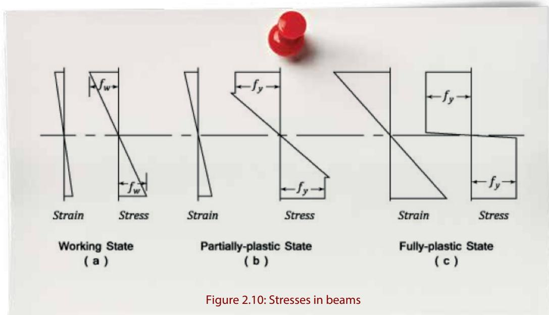
Figure 2.10: Stresses in beams
