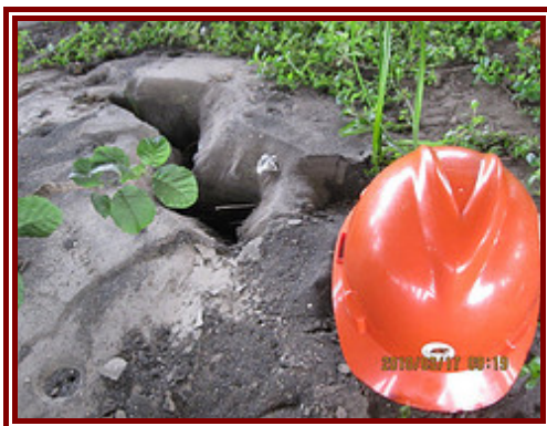
Figure 8-3: Evidence of liquefaction near the Bio-Bio River in Concepción. http://poweredbyorange.com/blog/
