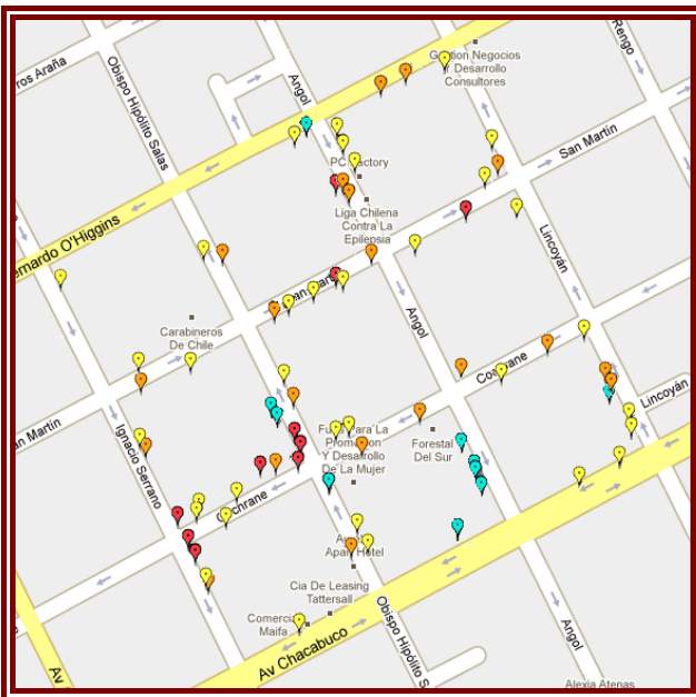
Figure 6-4: Block survey showing locations of damaged structures: Superficial damage (Yellow), Moderate Damage (Orange), Substantial or Very heavy damage (Red), Rubble on street (Blue).
