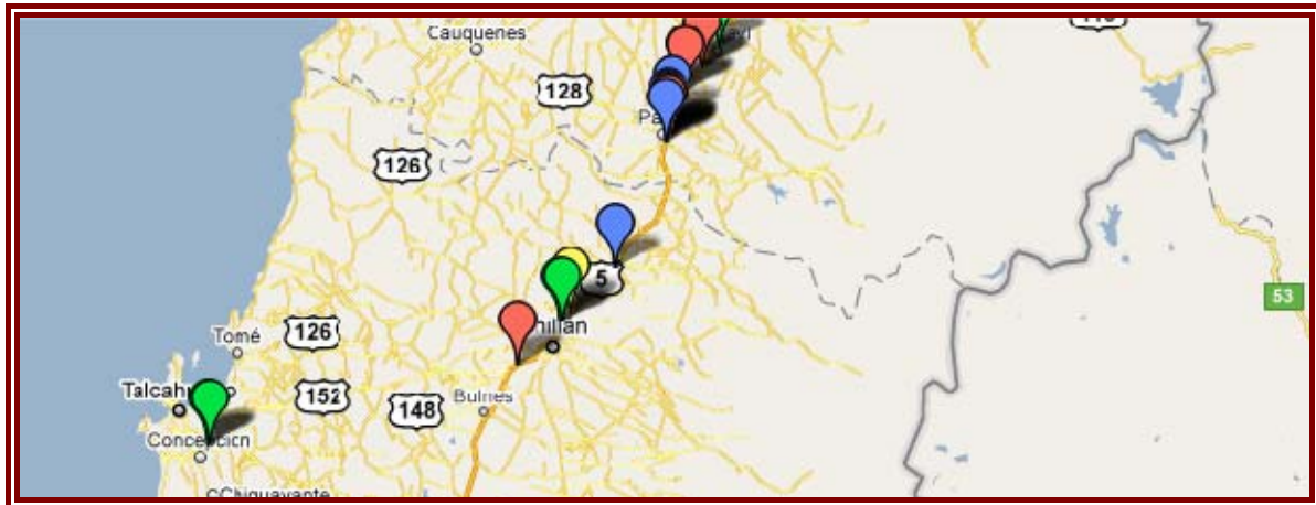
Figure 6-20: Bridge locations observed on the drive south. (Red – span(s) collapsed, Yellow - damaged, Green – appeared undamaged, Blue – severe settlement of road)
