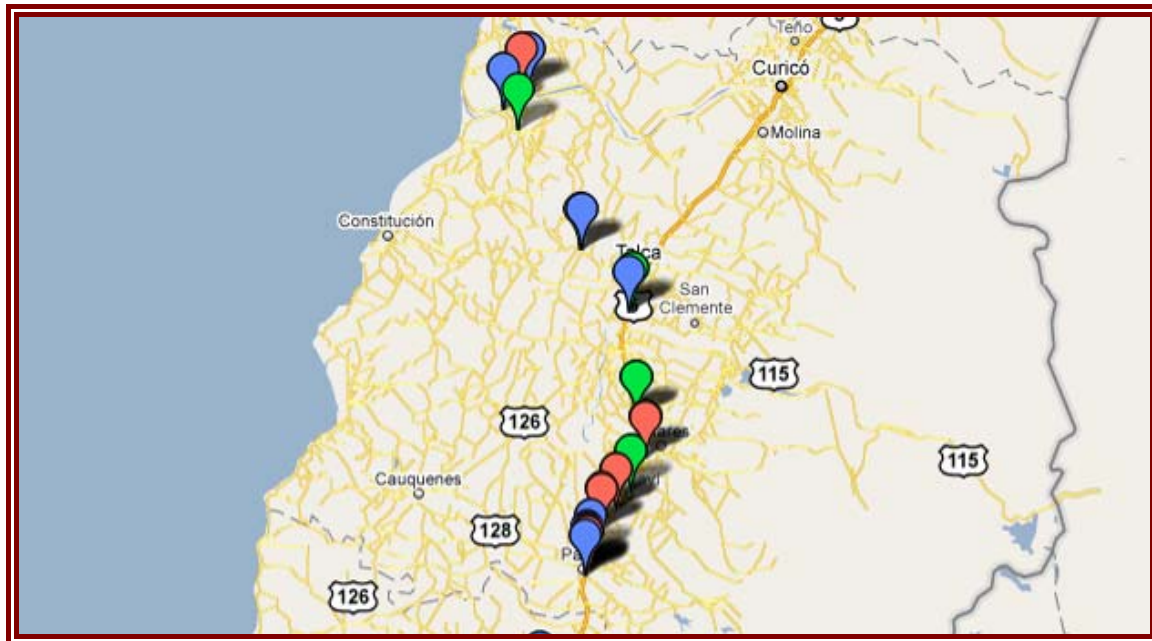
Figure 5-17: Bridge locations observed on the drive south. (Red – span(s) collapsed, Yellow - damaged, Green – appeared undamaged, Blue – severe settlement of road)
