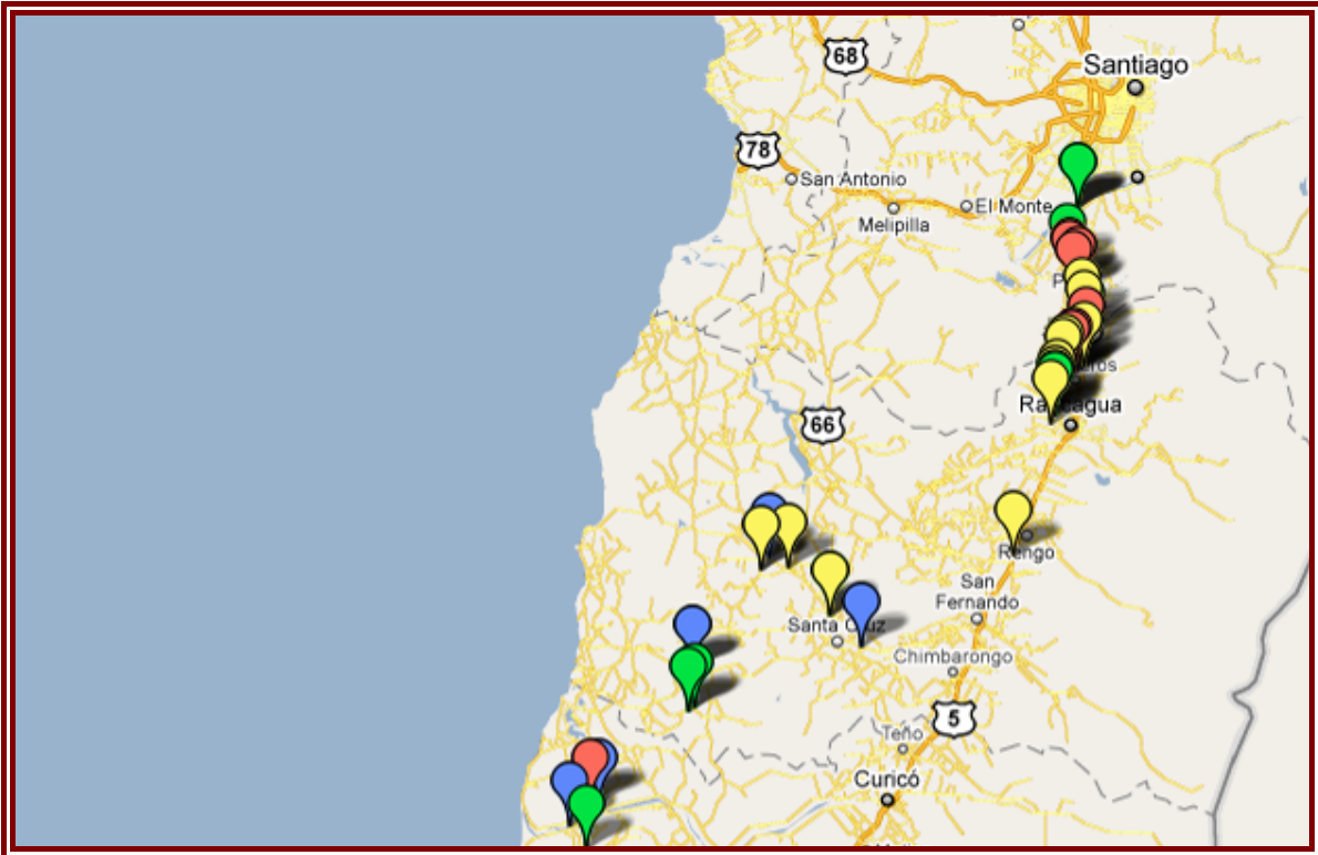
Figure 4-10: Bridge locations observed on the drive south. (Red – span(s) collapsed, Yellow - damaged, Green – appeared undamaged, Blue – severe settlement of road)
