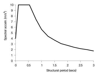
FIGURE Q8-2 : 475 year return period 5% damped spectrum for the region for rock with a wave velocity  $V_s$  of at least 800m/s at the surface
