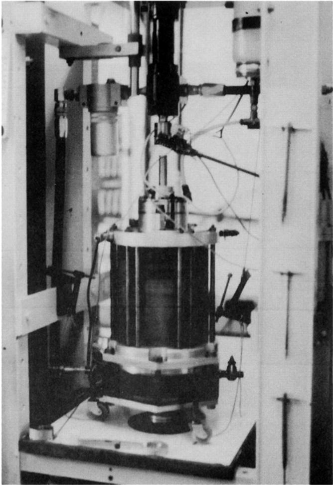
Clay sample in repeated loading triaxial apparatus
