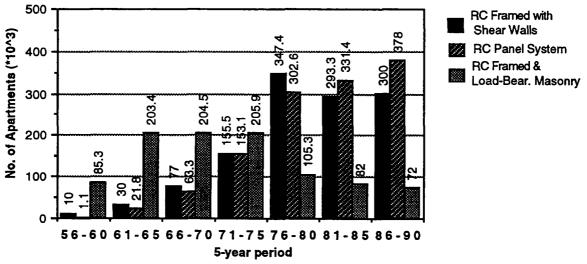
Figure 6: The construction of apartments by structural system during the 1956-90 period in urban areas of Romania.
