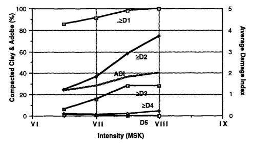
Figure 8: The vulnerability of low-rise compacted clay and adobe buildings (Bucharest, 1977 earthq.).
