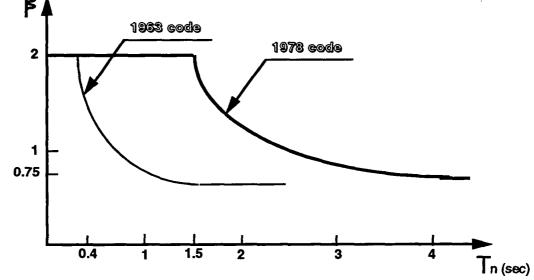
Figure 5: The effect of changes with the introduction of the 1978 code, upon the amplification factor ( $\beta$ ).
