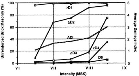
Figure 9: The vulnerability of low-rise unreinforced brick masonry buildings as revealed after a damage survey in Bucharest in 1977.
