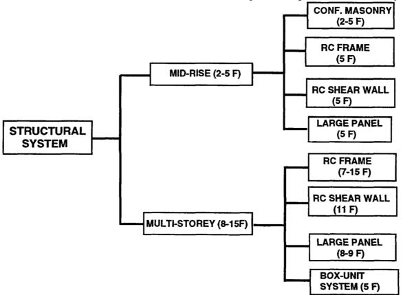
Figure 12: The building type distribution of state constructed large apartment buildings after1950 in Romania.
