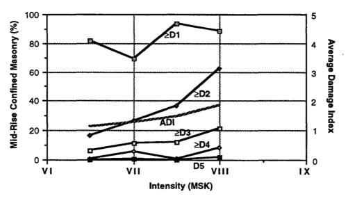
Figure 11: The vulnerability of mid-rise confined brick masonry buildings (Bucharest, 1977) .
