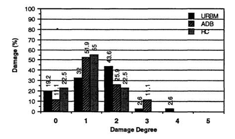
Figure 16: Damage degree histograms of the three main building types in the survey of Buzau (URBM = Unreinforced Brick Masonry; ADB = Adobe-Clay; RC = RC framed and RC shear wall).
