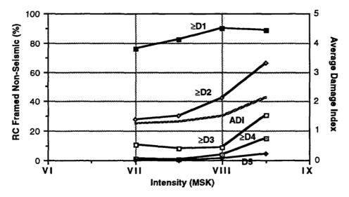
Figure 13: The vulnerability of the old RC framed apartment buildings (Bucharest, 1977 earthquake).
