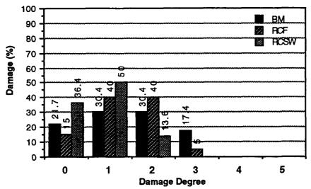
Figure 17: Damage degree histograms of the three main building types in the survey of Focsani (BM = Brick Masonry; ; RCF = RC framed; RCSW = RC shear wall).
