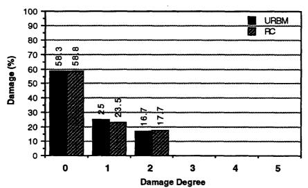
Figure 18: Damage degree histograms of the two main building types in the survey of Valenii de Munte (URBM = Unreinforced Brick Masonry; RC = Reinforced Concrete).
