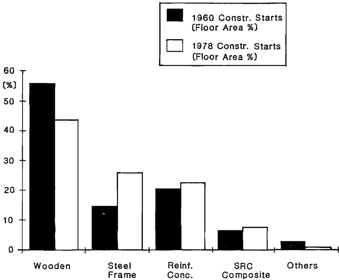
Figure 4.1 Proportion of building starts in Japan in 1960 and 1978, by structural type
