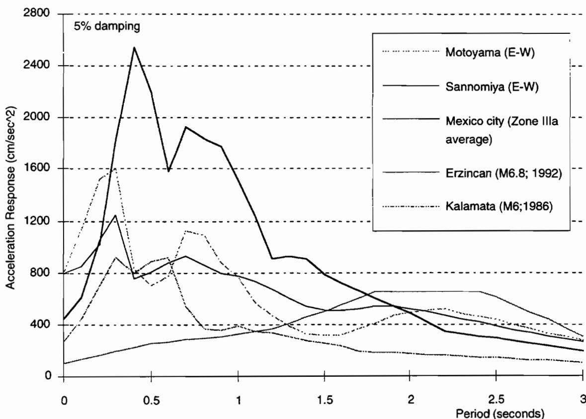
Figure 5.3: Response spectral accelerations (5% damping) in Sannomiya (JMA Kobe Kaiyo) and Motoyama (KOB Motoyama Primary School) compared to those of other recent destructive earthquakes. Their locations are shown in Figure 5.1.
