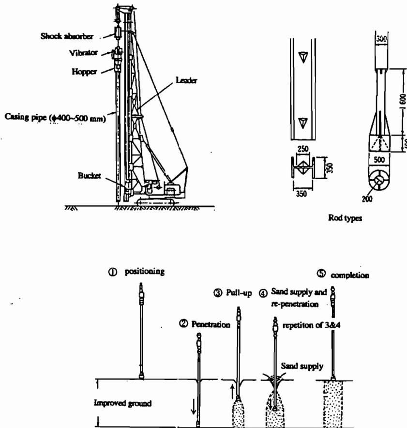
Figure 8.18 Ground improvement by the sand compaction pile method
