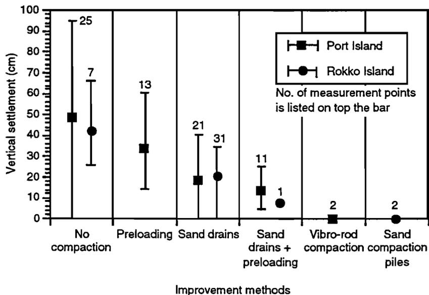
Figure 8.20 Measured vertical settlements at improved ground sites (after Mitchell, et al., 1995; Ishihara et al., 1995)
