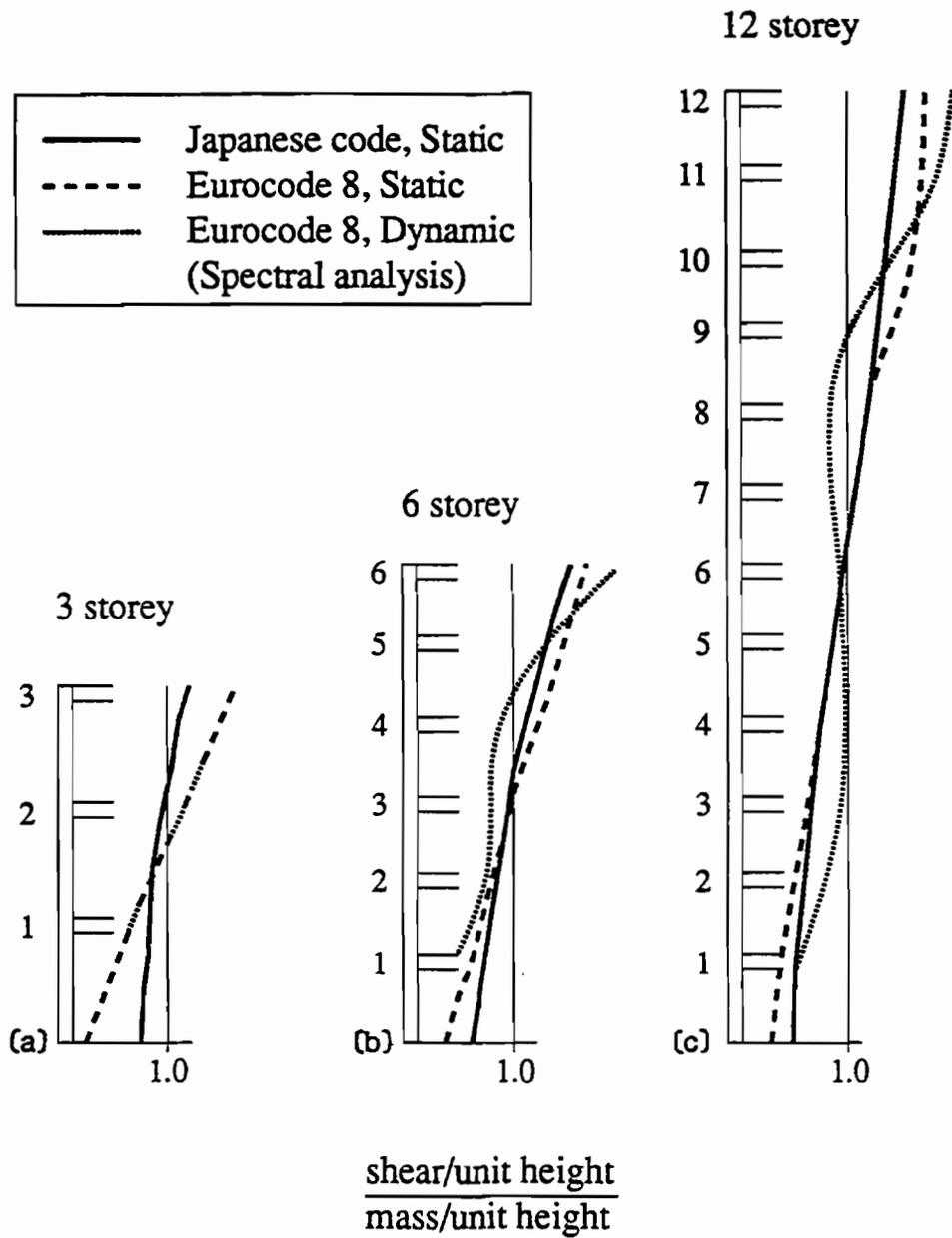
Figure 4.10 Comparison of distribution of lateral loading in present Japanese design and Eurocode 8
