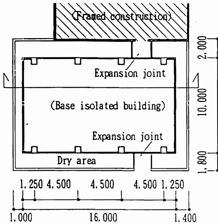
Figure 4.6a A plan of the first floor of the MTRC base-isolated building
