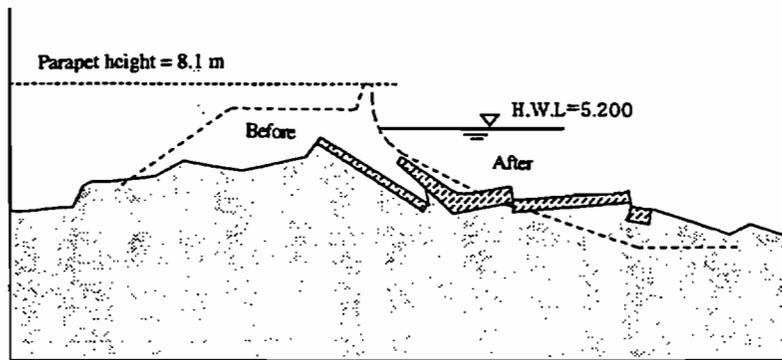
Figure 8.28 Failure of river dykes along the Yodo river (JSCE, 1995)
