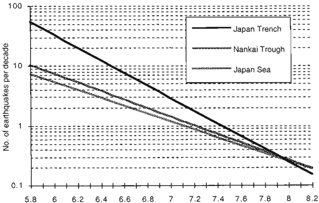
Figure 2.2: Magnitude and frequency of occurrence relationship in Japan seismicity zones
