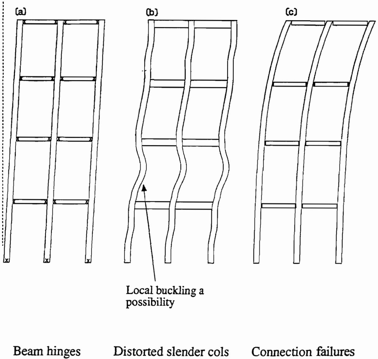
Figure 4.13 Deformed shapes of damaged buildings
