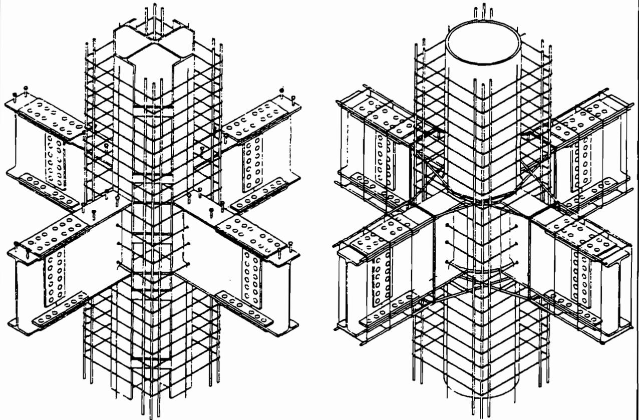
Figure 4.3 Typical beam/column joints in SRC construction
