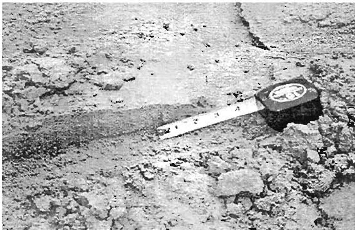
Plate 8.3: A layer of liquefied sands erupted from the ground
