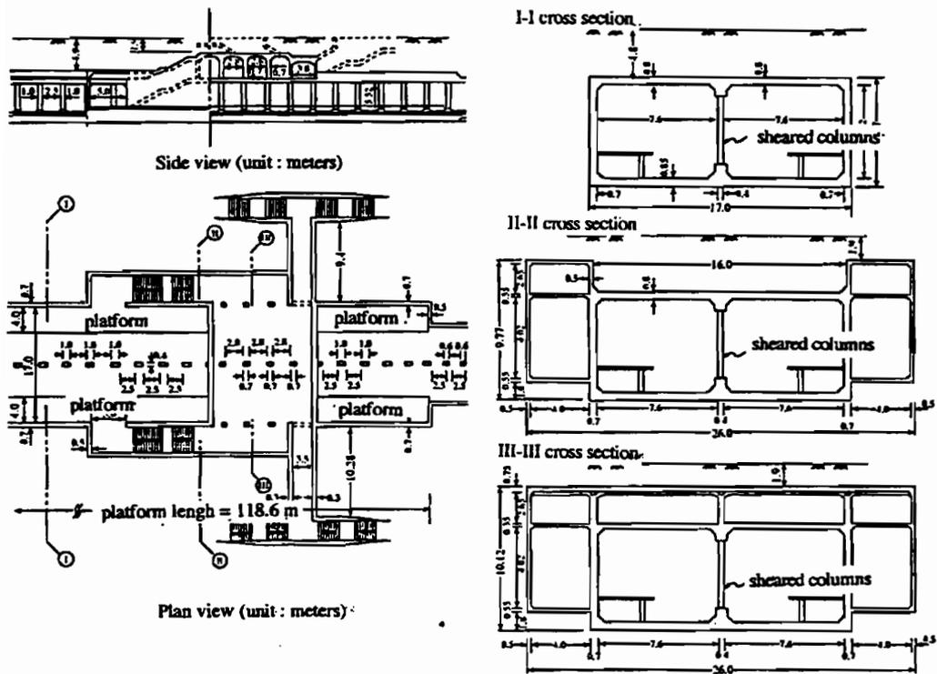
Figure 8.22 Cross-section of the Daikai station
