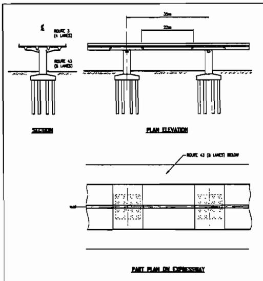
Figure 2 Typical Arrangement of the 635m Long All-Concrete Section of the Hanshin Expressway which Collapsed
