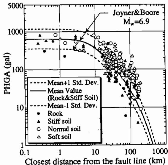
Figure 3.10 Attenuation of peak horizontal ground acceleration (Ejiri et al., 1996)
