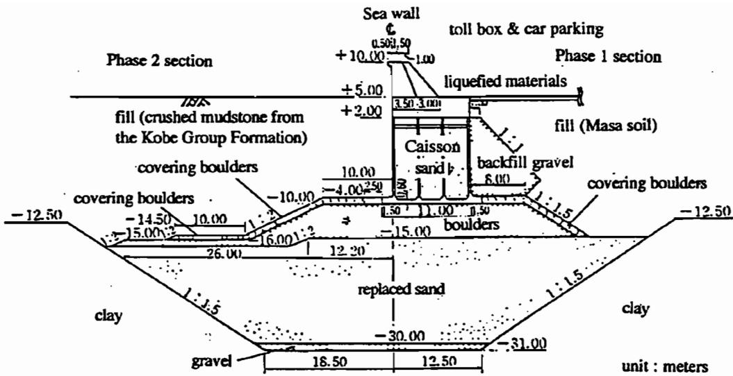
Figure 8.8 Cross-section of the caisson walls between Phase 1 and 2 of Port Island (Konoike, 1996)
