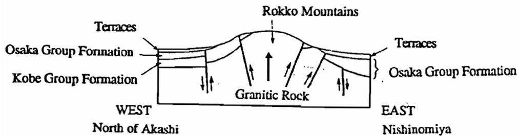
Figure 3.4 Schematic diagram of geographic features of the Kobe region
