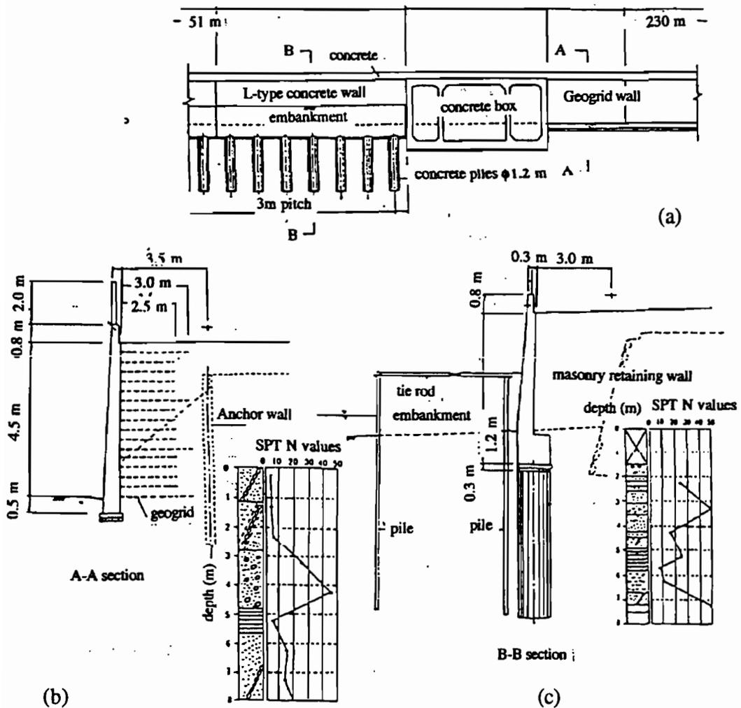
Figure 8.26 Cross-sections of the retaining walls at Tanata (Tatsuoka et al., 1995)
