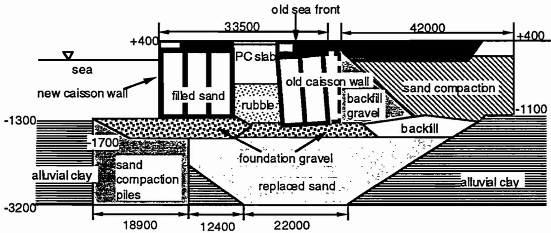
Figure 8.9 Cross-section of a new quay wall on the south section of Rokko Island (Wako, et al. 1996)
