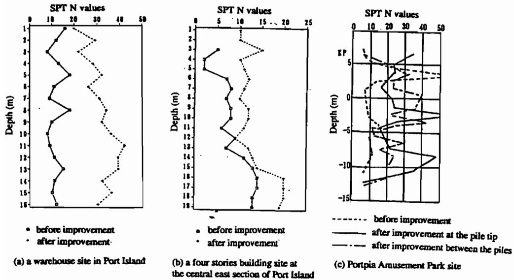
Figure 8.17 SPT N-values before and after the ground improvement (Fudo Construction, 1995)
