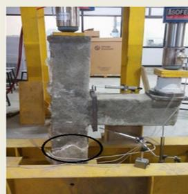
Figure 4. Crack pattern with FRP wrapping.
