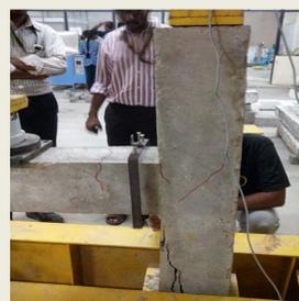
Figure 1. Crack pattern without FRP wrapping.
