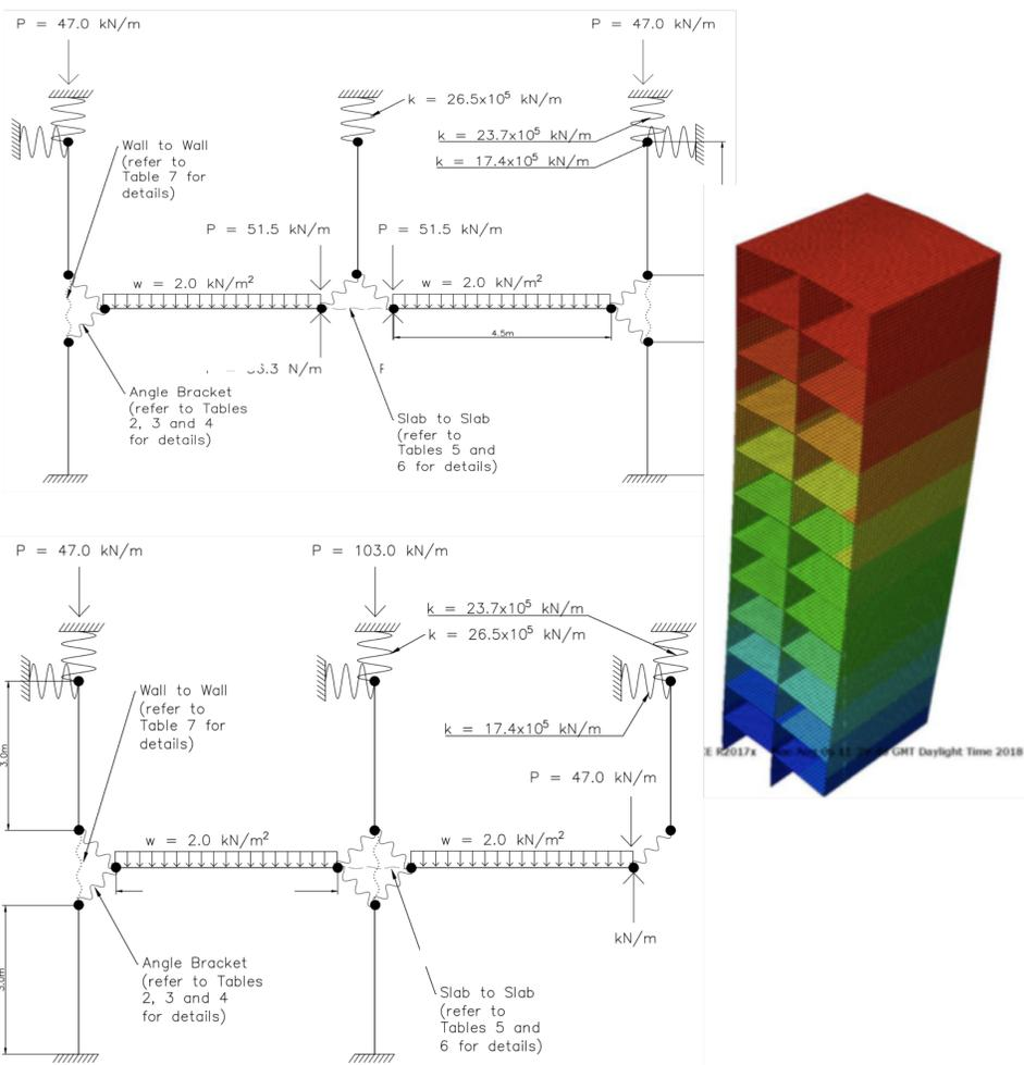
Two scenarios were studied, one where the main floor interior wall was assumed to fail (top left), and the other where a main floor edge wall was assumed to fail (top left). The floor loading seen in the figures was determined by means of static analyses. Global models (right) were also employed to verify the dynamic response of the building.
