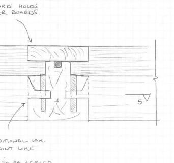
210W × 24 THICH BOAM NOTCHED BOARDS SLEEWED DOWN BOARD. NAILED? TO LANDING BEAM DIMS AS 120.01 ALL SIDE TIMBER FIXED TO THE WITH THROUGH BOLTS IN PELLETED MOLES.
