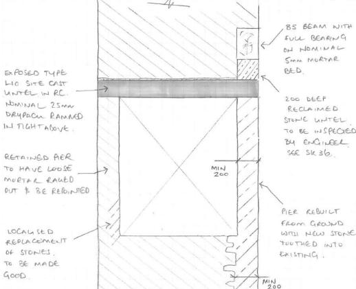
, BS BEAM WITH FULL BEARING ON NOMINAL SMM MORTAR BED. 200 DEEP RECLAIMED
