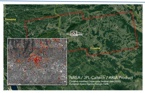
Figure 5-9 – The detail of the damage proxy map (DPM) interpreted by a team at Caltech and funded by NASA and the full extent of the analysed area (in the red polygon). The full map is available at:
