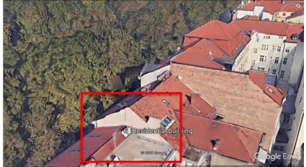
Gable failure of a residential building. The damage is contained within the upper part of the façade bounded by the red box
