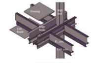
(a) Typical CFS modular framing
