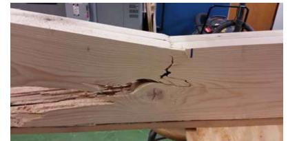
An example of a softwood and bamboo hybrid beam failing after a bending test (Kaboli and Clouston 2019).
