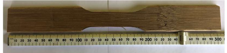
An unjointed specimen with a thinner central gauge section, specimens without a splice were tested so the performance of the joints could be directly measured.
