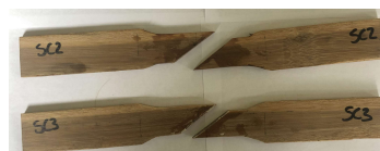
Failure of scarf joints with both adhesive types
