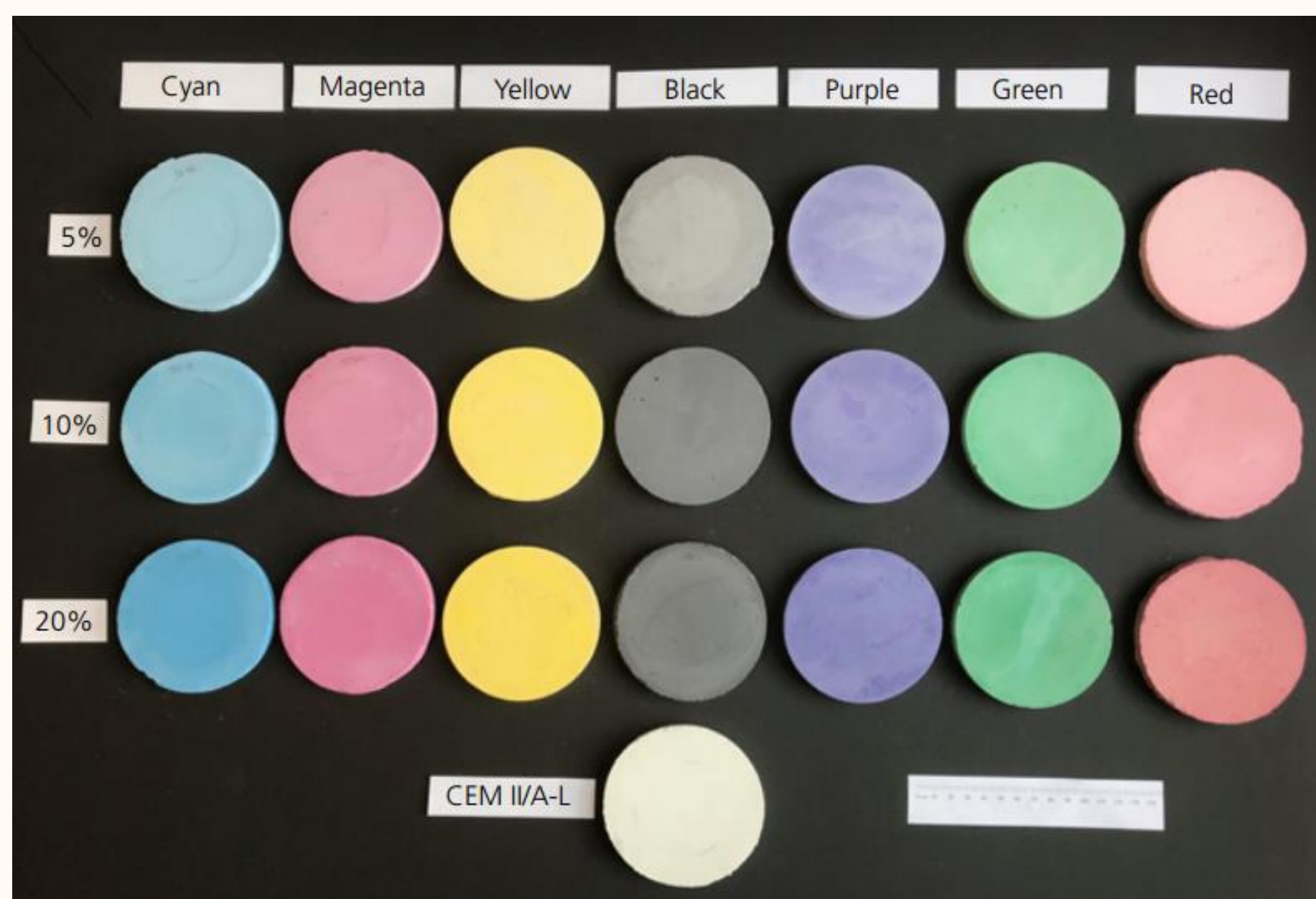
Range of concrete colours possible using recovered toner ink (Newlands, et al, 2018)
