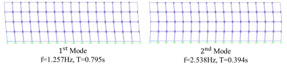
■ The dynamic structural behaviour of the modular building conformed to a typical single-degree-of-freedom cantilever structure.
