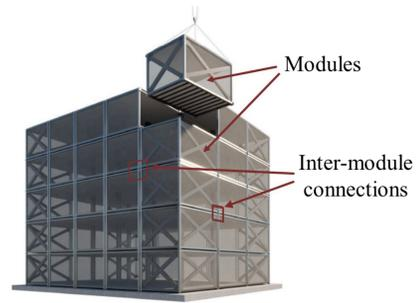
Construction of modular building [1] Modular steel building [2]
