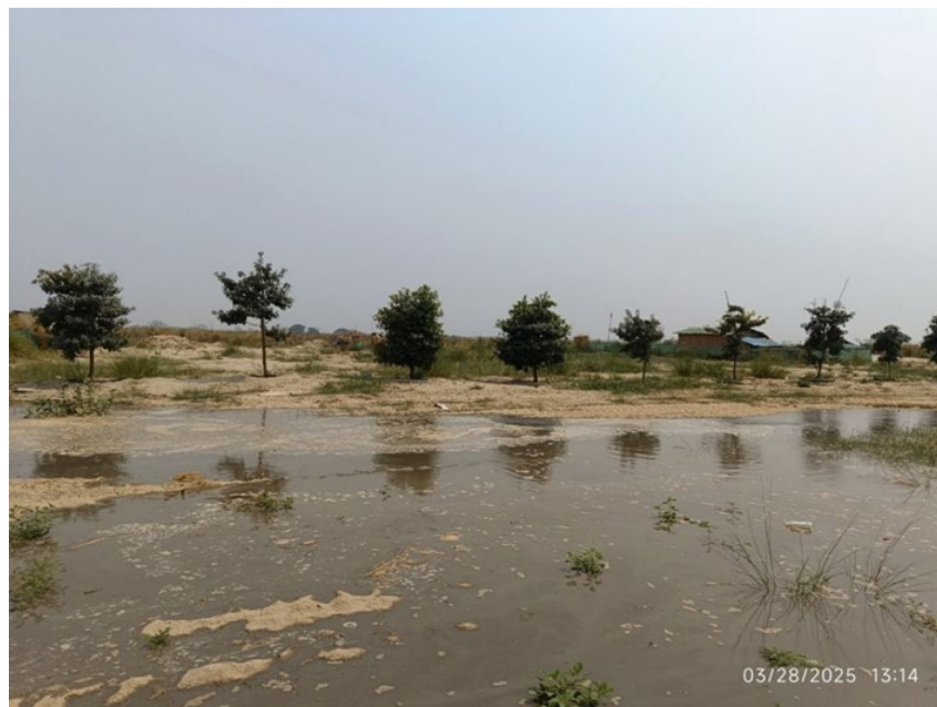
Figure 4.6.3. Liquefaction ejecta post-earthquake in area where ground improvement work for Amarapura Urban Development Project had not yet been completed (Credit: ZoMung Thawng).
