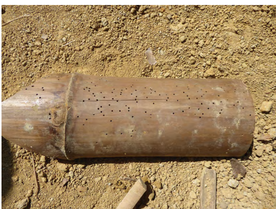
a) Beetle exit holes visible on side of bamboo
