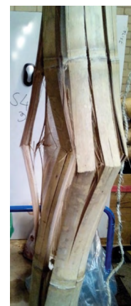
Figure 6.5: Axial failure of G. Angustifolia culm 6.5
