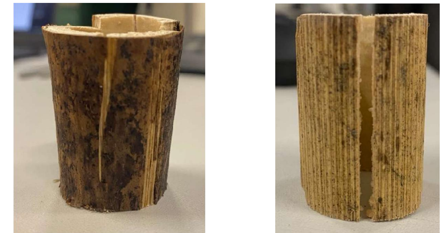
Figure 6: failure modes of shear tests
