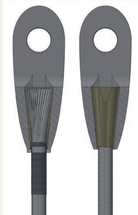
FIGURE 7: Casting of socketing material around brush within end connection
