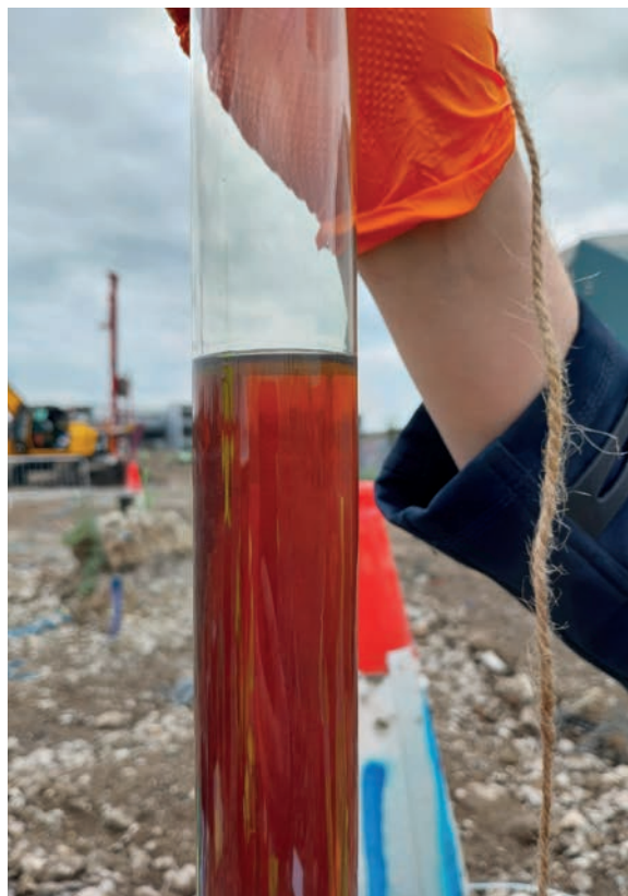
FIGURE 3: Light non-aqueous phase liquid recovered from borehole
