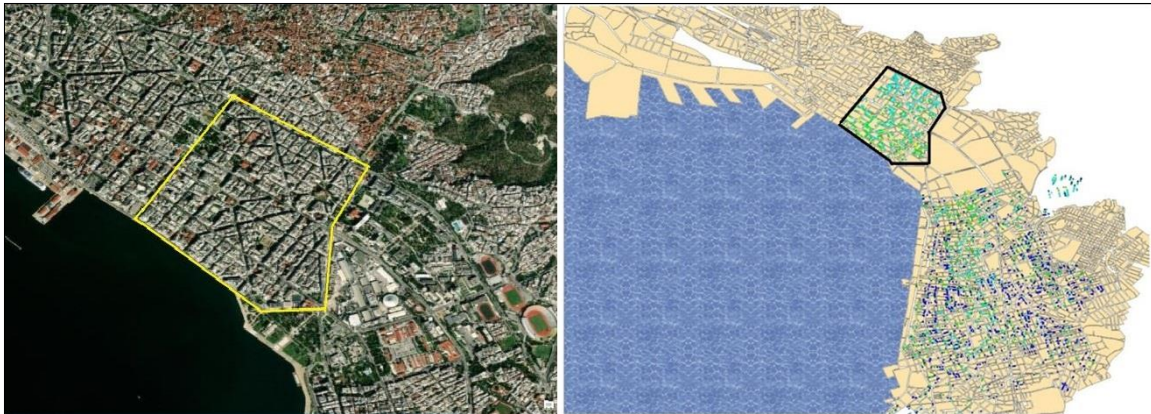
Figure 12: Study area (left) and reported damage to 3,707 RC buildings during the 20 June 1978 Thessaloniki earthquake (right), based on Panou et al. (2014).
