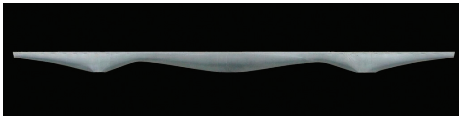
Figure 8 Fabric-cast concrete 'bending moment' beam
