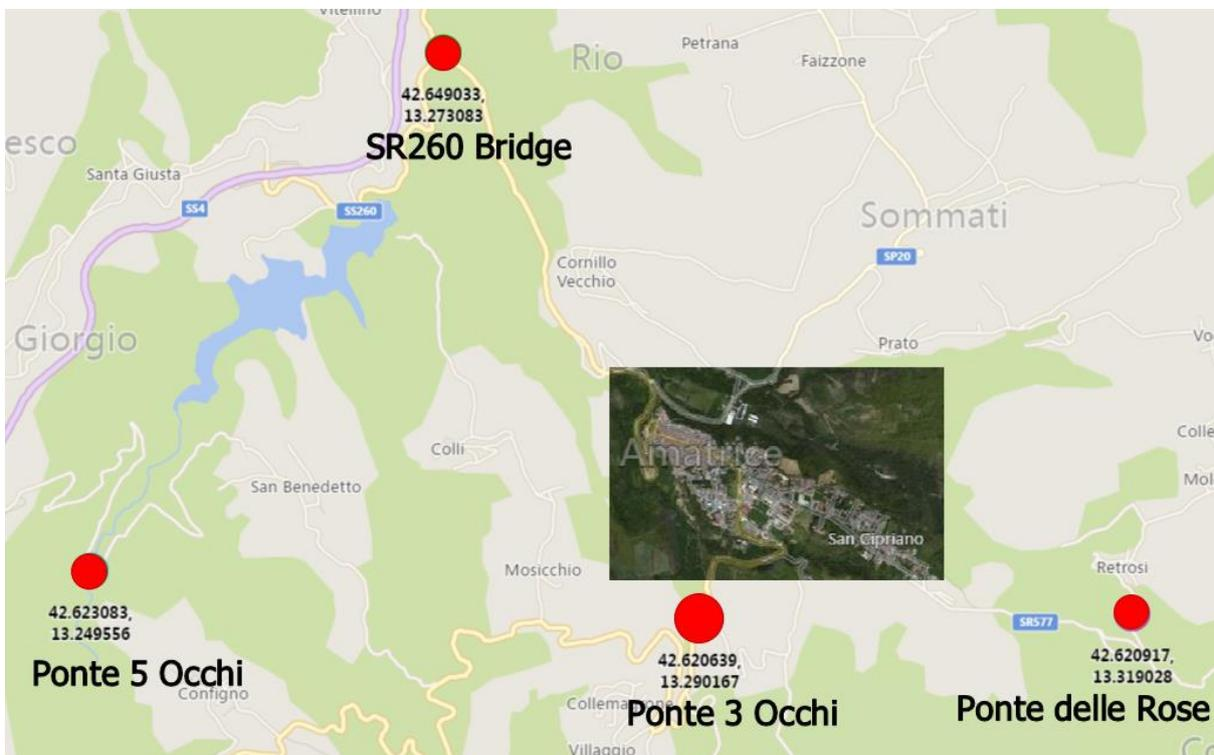
Figure 8-2 Amatrice plan view, showing the access roads and the bridges inspected (background map from maps.google.co.uk).
