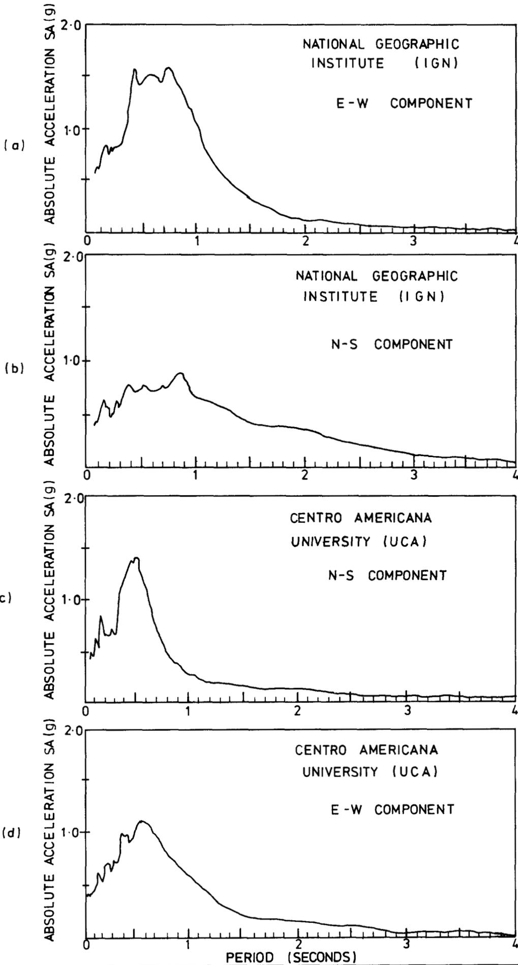
FIGURE 15: RESPONSE SPECTRA OF ABSOLUTE ACCELERATION FOR 5% DAMPING, FROM HORIZONTAL STRONG MOTION RECORDS AT THE NATIONAL GEOGRAPHIC INSTITUTE AND THE CENTRO AMERICANA UNIVERSITY.
