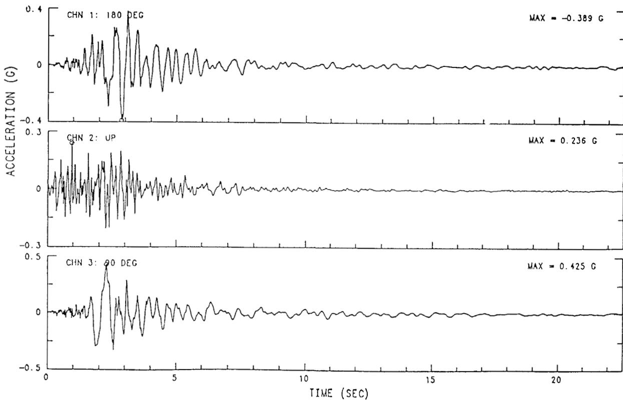
FIGURE 11 : UNCORRECTED STRONG MOTION RECORDS FROM THE BASEMENT OF THE CAMINO REAL HOTEL (HCR).
