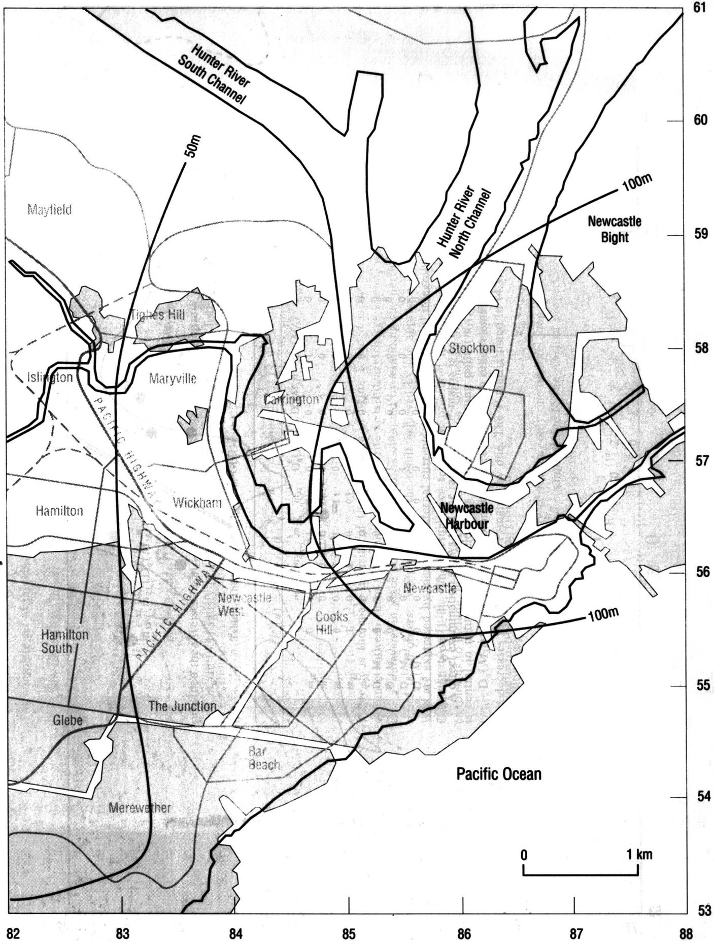
**Boundaries of coal extraction and contours to base of borehole seam**
