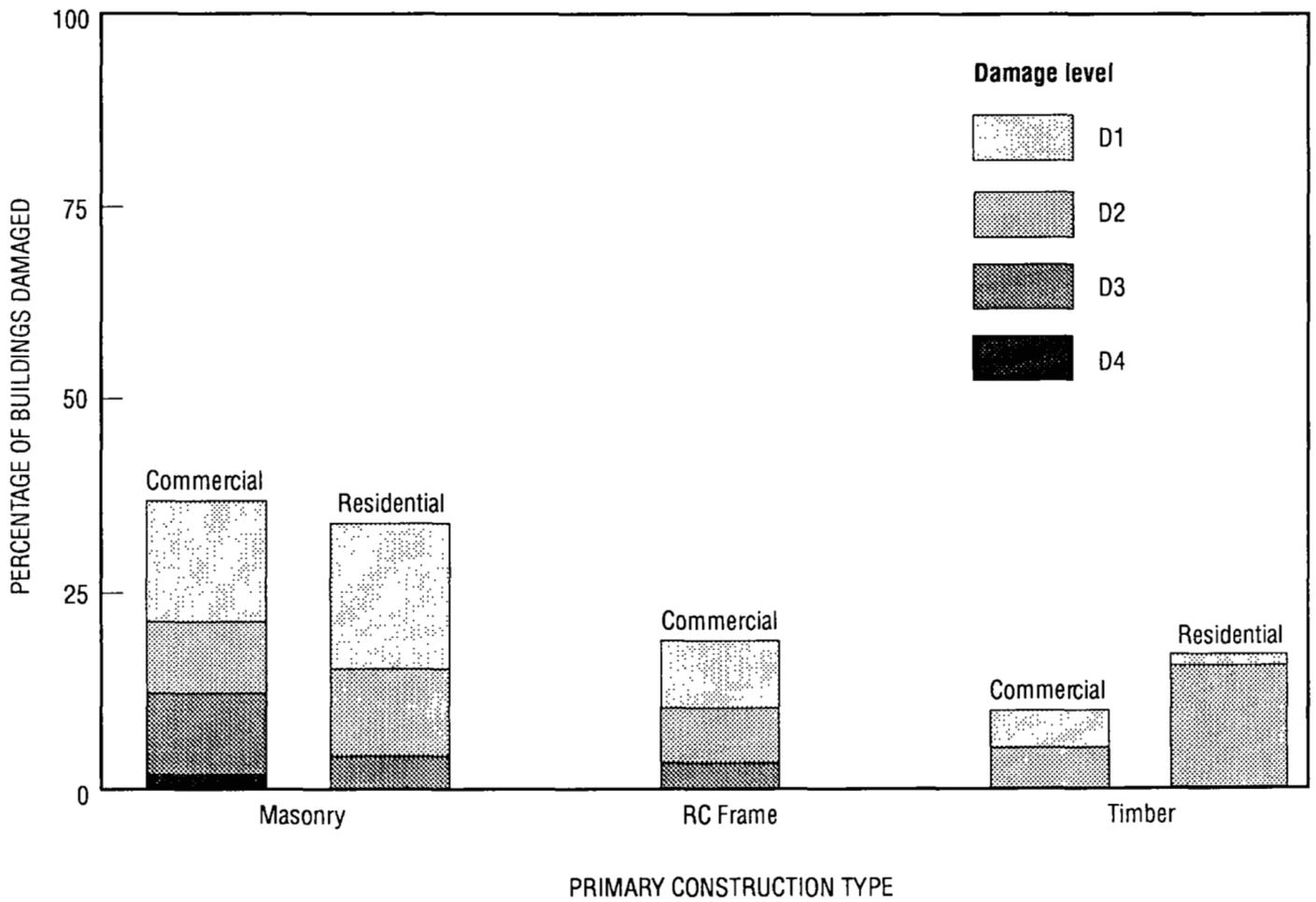
**Variation of damage levels with primary construction type and use**
