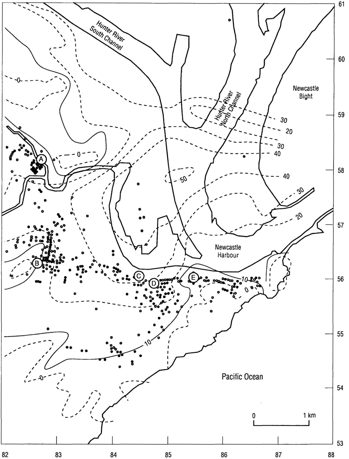
Distribution of damage in relation to soil thickness
