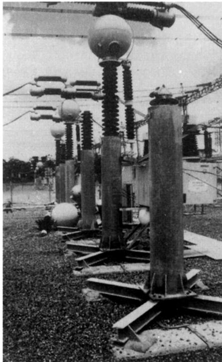
PLATE 5.76 *Failure of porcelain insulators supporting 132kV circuit breakers at Killingworth, 20km west of Newcastle*
