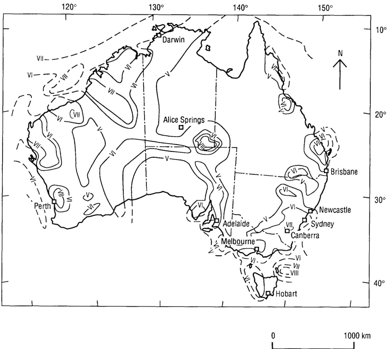
**Intensity (modified Mercalli scale) with a 10% chance of being exceeded in a 50 year period (after Gaul et al 1990)**
