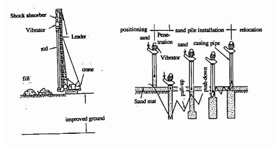
Figure 8.16 Ground improvement by the vibro-rod method
