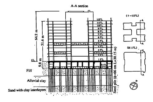
Figure 8.12 Pile foundation of the Kobe Shimin Hospital
