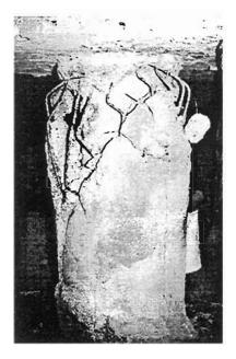
Plate 8.20: Damaged pile foundation due to soil liquefaction (photo by Prof. K. Tokimatsu)
