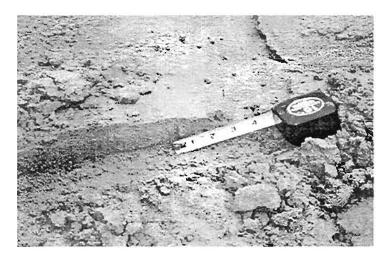
Plate 8.3: A layer of liquefied sands erupted from the ground
