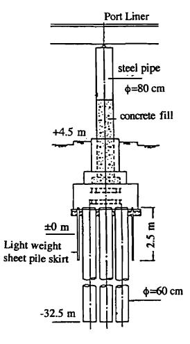
Figure 8.13 Pile foundation of the elevated Portliner Railway on Port Island (Watanabe, 1981)
