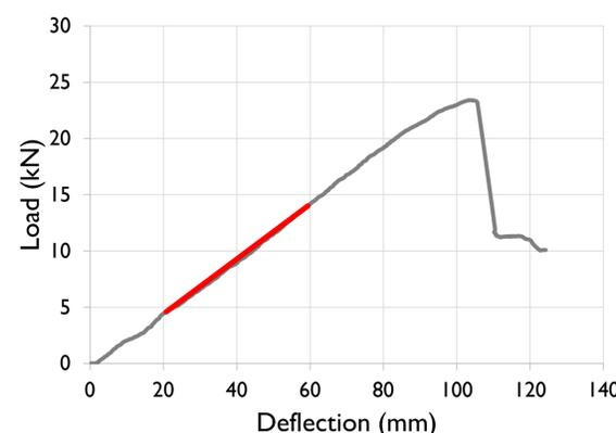
Specimens were loaded at a rate of 0.5m/s and deflection was measured at the mid-point and supports.
