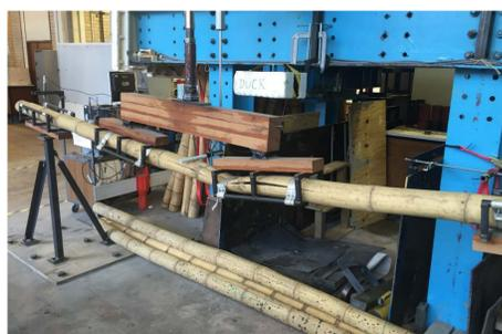
A four-point bending test was then conducted to determine the Static Modulus of Elasticity, the Modulus of Rupture (strength) and the bending moment capacity of each specimen. The test configuration is shown to the left.
