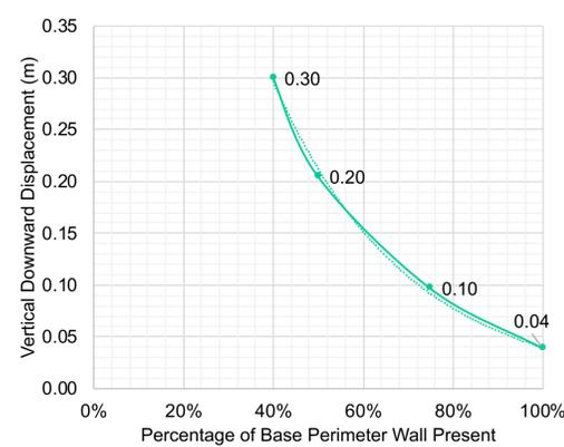
A sensitivity study on the percentage of the main floor perimeter walls present (with the removal taking place from the bottom upward) was conducted. This was completed with rotationally and translationally rigid connections. The support load removal time interval was 0.01s.
