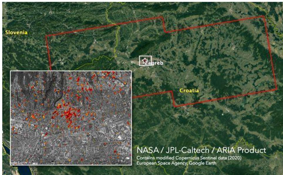
Figure 5-9 – The detail of the damage proxy map (DPM) interpreted by a team at Caltech and funded by NASA and the full extent of the analysed area (in the red polygon). The full map is available at: <https://maps.disasters.nasa.gov/arcgis/home/webmap/viewer.html?layers=db20d487cee24810bd7b8cc96ccb3b>
