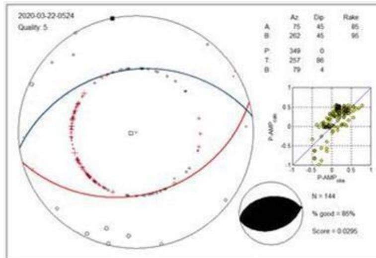
Figure 3-10 – Focal mechanism of the main shock calculated with the direction and amplitude of the first P-wave displacement taken from the 144 seismograms recorded in Croatia and across Europe.
