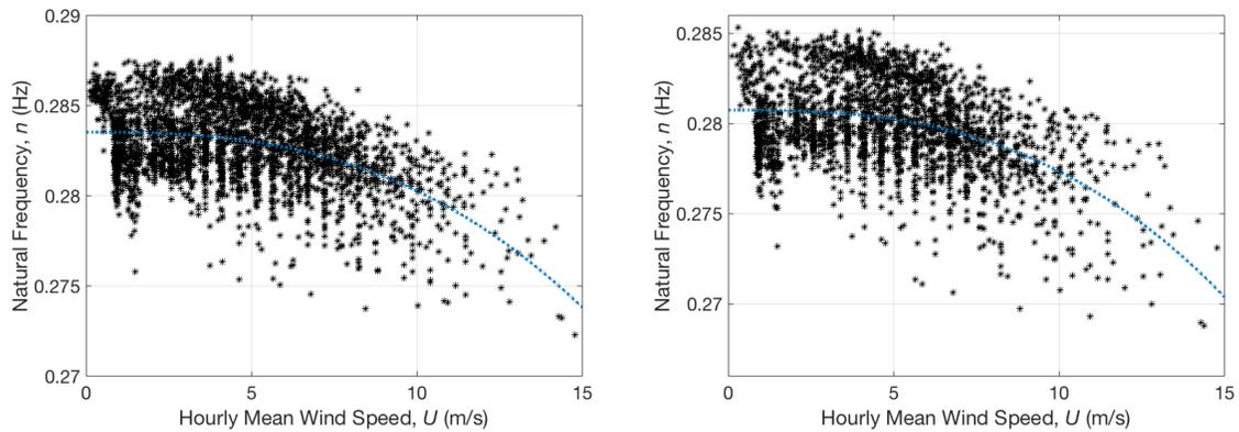
Figure 7. Relationship between first natural frequency and the corresponding 1-hour mean wind speed in the x (left hand-side plot) and y directions (right hand-side plot).
