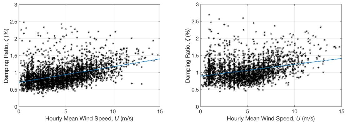
Figure 5. Relationship between damping ratio of the first mode and the corresponding 1-hour mean wind speed in the  $x$  (left hand-side plot) and  $y$  directions (right hand-side plot).
