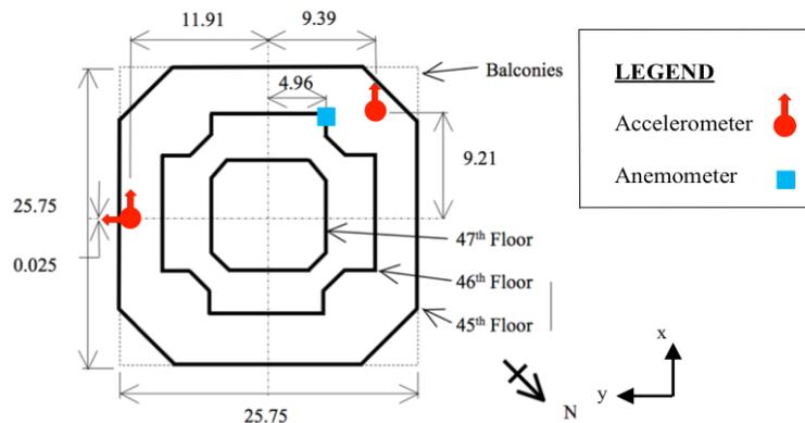
Figure 1. Plan of the top three floors of tower showing locations of instruments and local coordinate system (dimensions in m).
