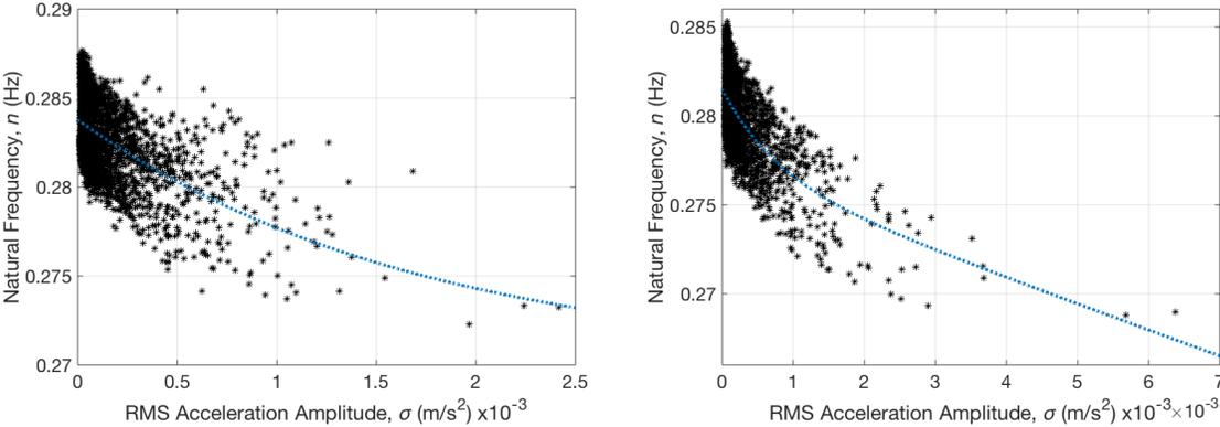
Figure 8. Relationship between first natural frequency and the corresponding RMS acceleration amplitude in the x (left hand-side plot) and y directions (right hand-side plot).
