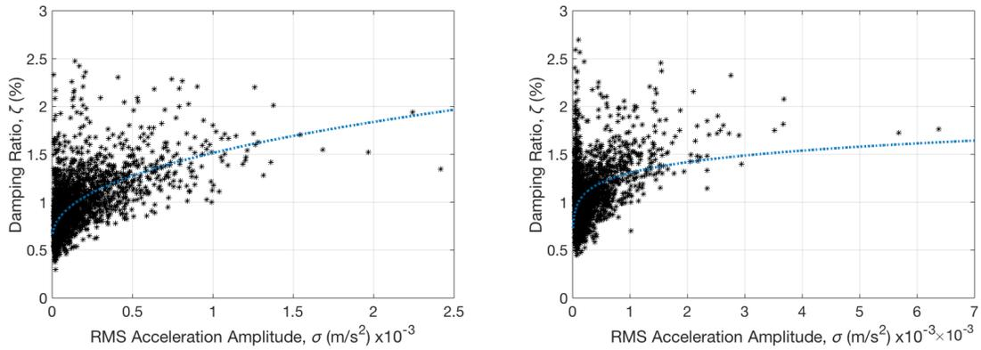
Figure 6. Relationship between damping ratio of the first mode and the corresponding RMS acceleration amplitude in the x (left hand-side plot) and y directions (right hand-side plot).
